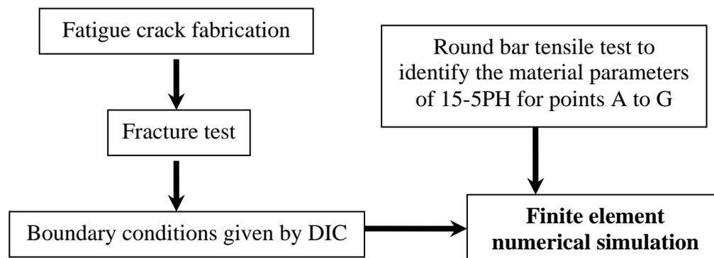
Fig. 3.1 The methodology to get  $J_{IC}$  from experiments
