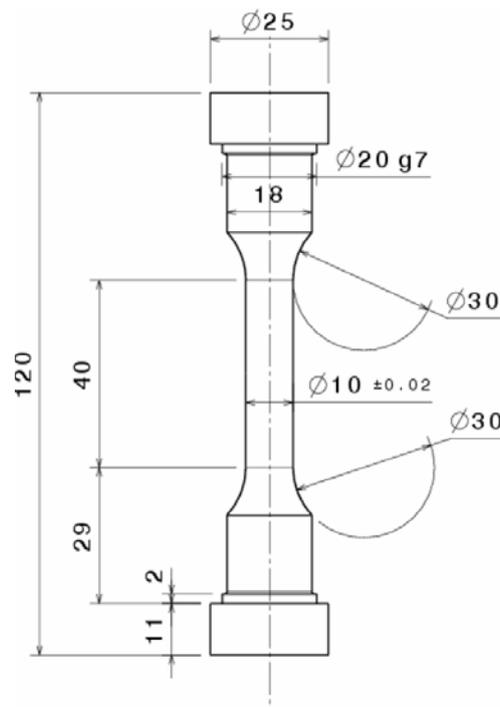
Fig. 4.1 15-5PH round bar sample for tensile tests
