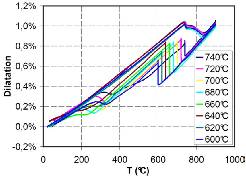
Fig. 5.3 Free dilatation curves of the isothermal transformation at temperature higher than Bc
