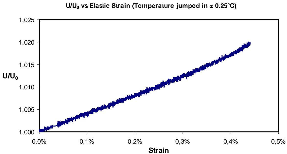
Fig. a13 Elastic strain induced potential drop
