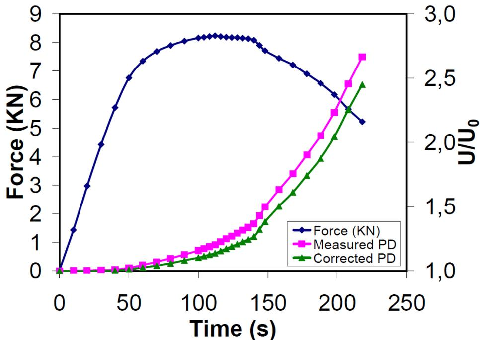
Fig. 3.3 Fracture test and potential drop acquisition
