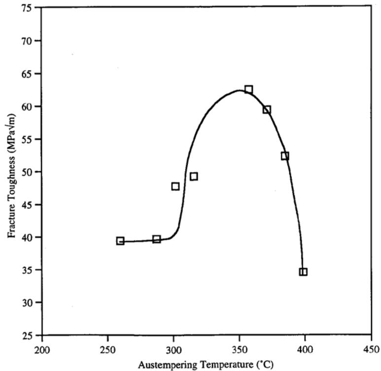
Fig. 2.24 Influence of austempering temperature on the fracture toughness of HCHS steel [91]
