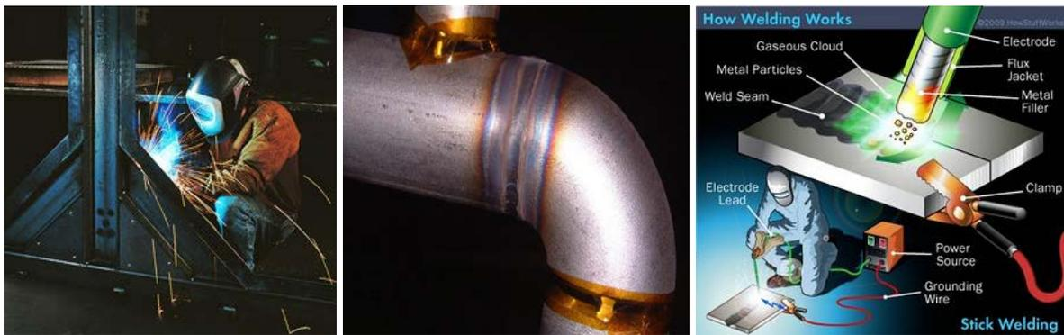
Fig. 1.1 Industrial crack reparation: welding [1-3]
