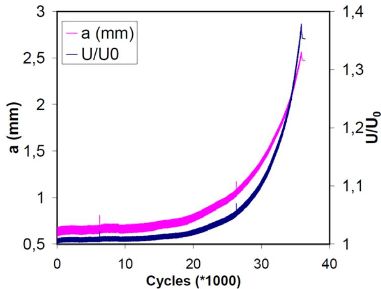
Fig. 2.6 Fatigue crack controlled by potential drop technique
