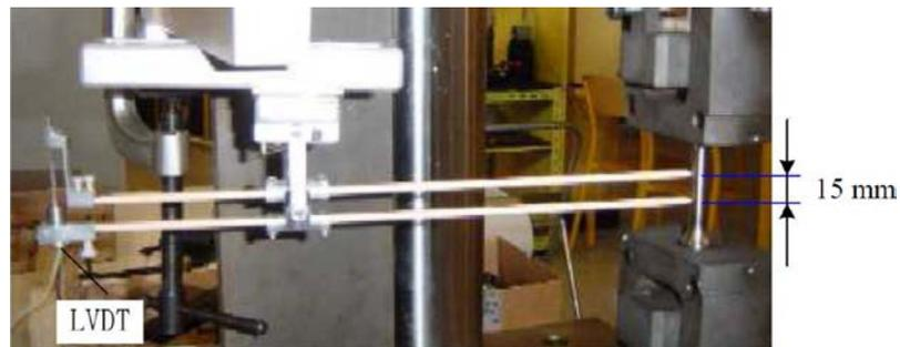
Fig. 4.2 Extensometer with 15mm distance between two sticks
