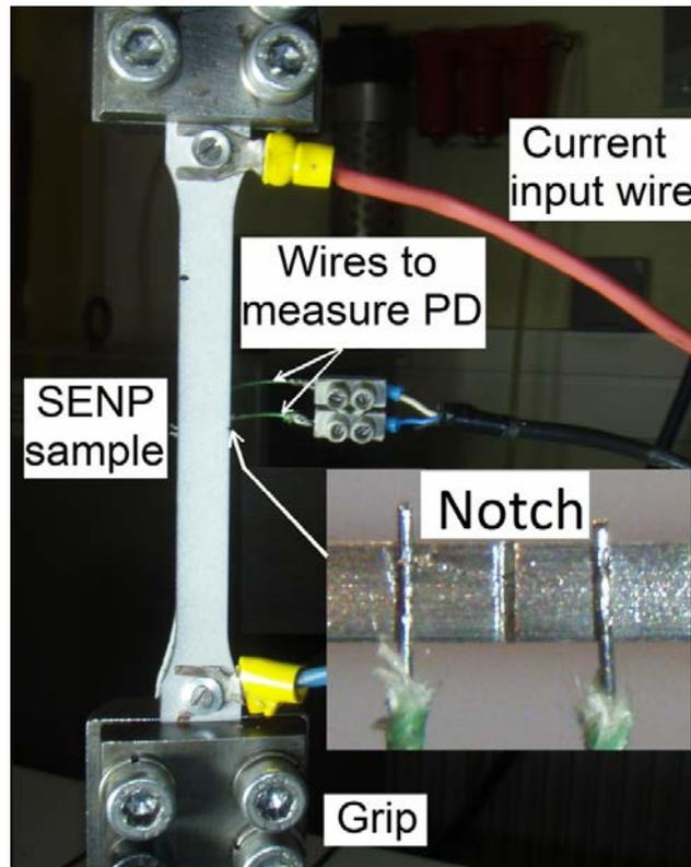
Fig. 2.5 Set-up of DC potential drop method
