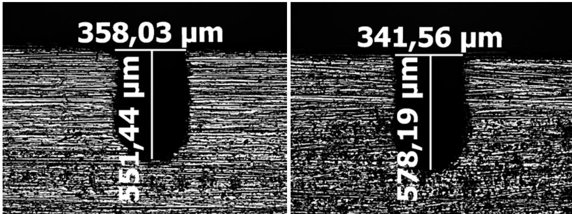
Fig. 2.4 The notch size from the views of two faces
