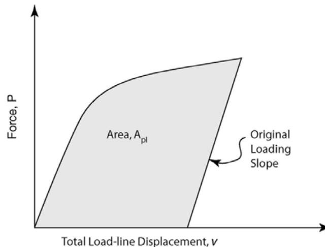
Fig. 2.37 Definition of area for  $J$  calculation using the basic method [139]
