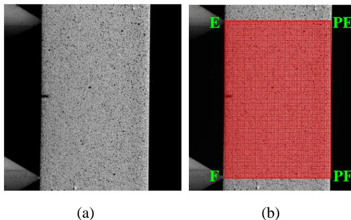
Fig. 3.6 Initial photo and ZOI during DIC process
