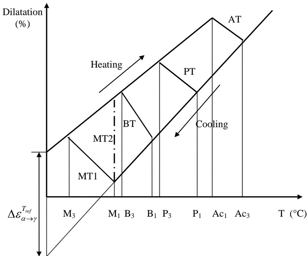
Fig. 2.2 Ideal schematic of dilatation curve during all kinds of transformations
