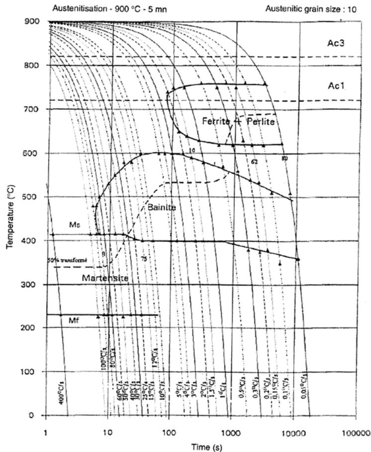
Fig. 2.19 CCT diagram of 16MND5 steel [44]
