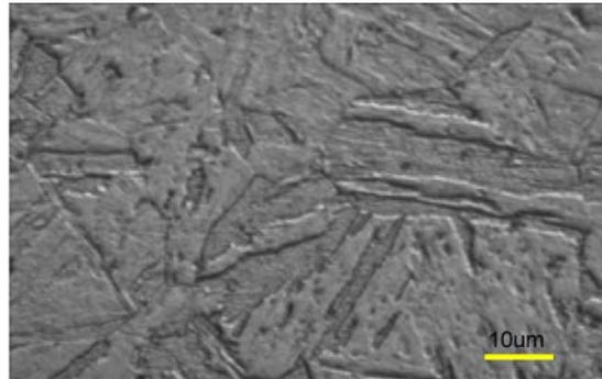
Fig. 2.13 Micrography of as received 15-5PH stainless steel [22]
