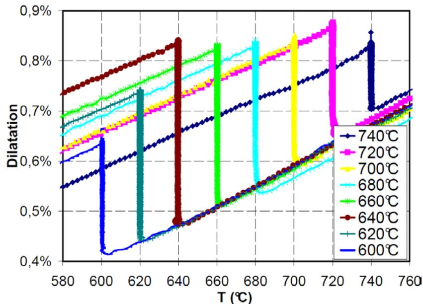
Fig. 5.4 Magnification of the free dilatation curves of the isothermal transformation at temperature higher than Bc
