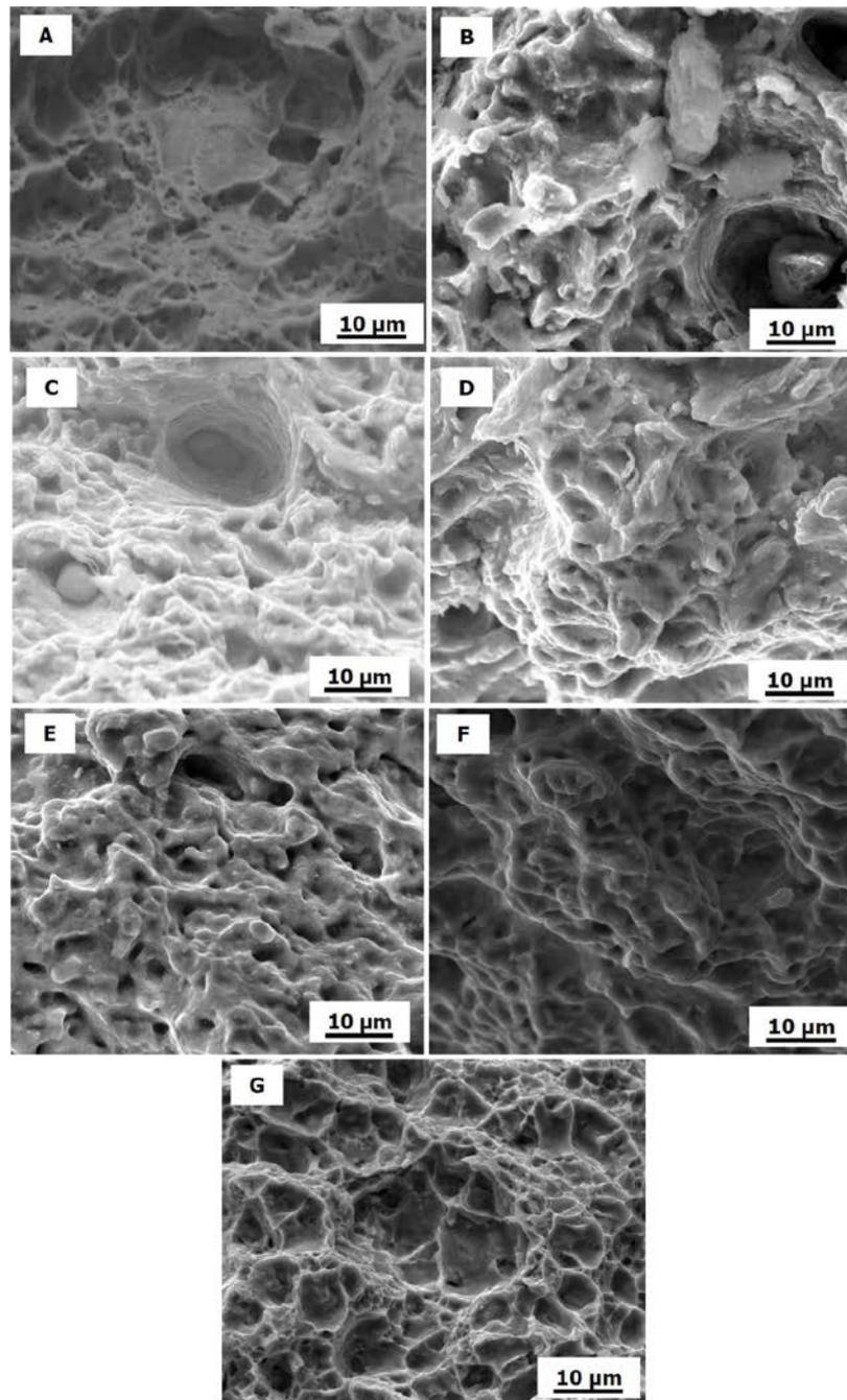
Fig. 5.29 Fractography of 16MND5 at different condition
