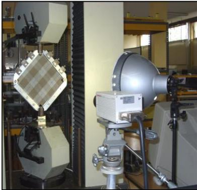
Figure 2.48: Essai de picture frame
