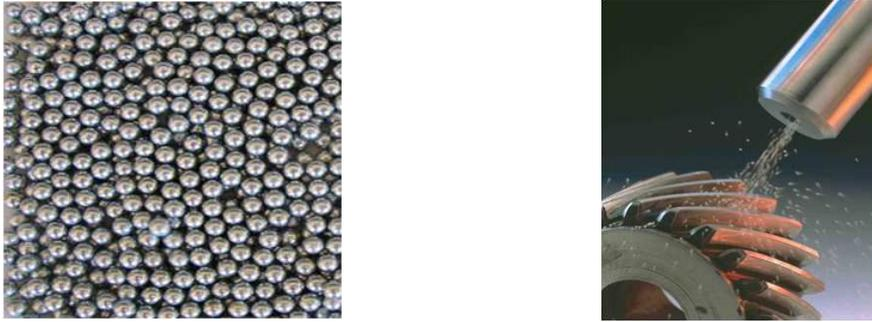
**Figure 1.10:** Shots (left) bombarding an helicoidal gear (right)
