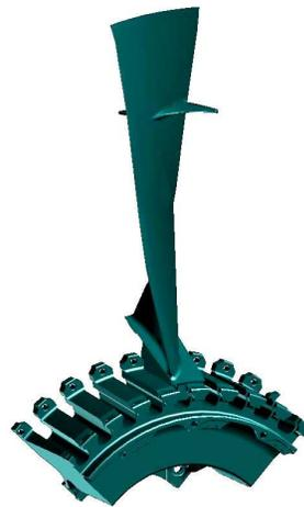
**Figure 1.3:** Blade and disk linked together using a dovetail joint
