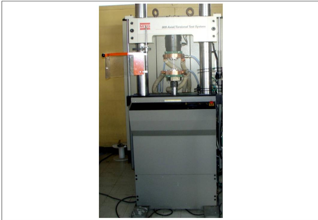
**FIGURE 2.9:** Machine de traction / compression - torsion MTS 809
