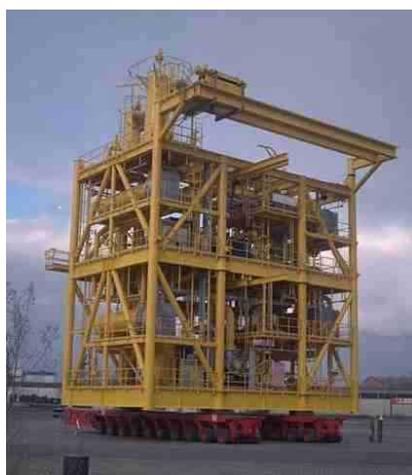
Figure 4.3 – Module de compression
