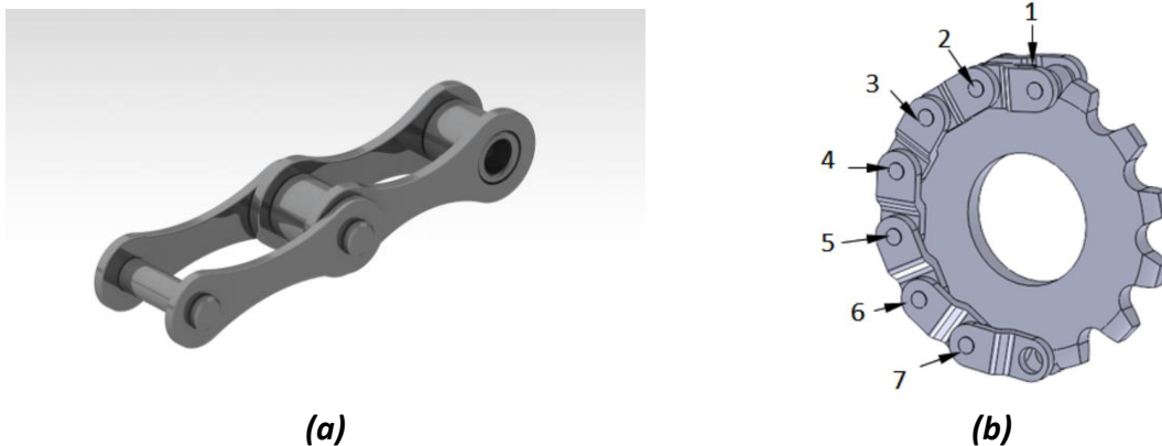
Figure I-3: (a) Double pitch chain (b) Cranked link chain [12]
