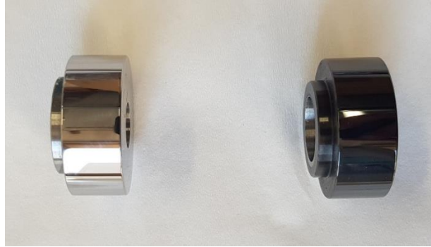
Figure 2.5: Uncoated steel barrel (left). DLC-coated steel barrel (right).
