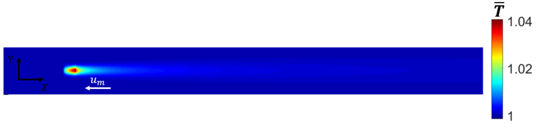
Figure C.2: (X, Y) plane of the liner surface with a moving heat flux
