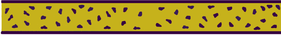
Figure 101. New sample MG-H-86 with a bi-disperse mixture between matrix particles and 50 angular grains homogeneously distributed and of the same equivalent diameter ( \Phi_{eq} = 315 \mu m ). (MG-H-86, for Matrix-Grains sample with Homogeneous distribution and 86% of matrix particles)
