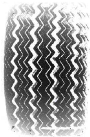
Figure 7.2: The profile obtained by using the Fringe Projection Method (FPM) on a trailer tire 5.2S10 [MAN 19b].
