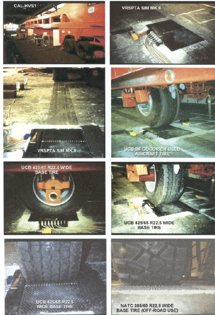
Figure 1.7: Images of the Vehicle Road Surface Pressure Transducer Array(VRSPTA) SIM MK II system during the UCB/NATC tests. [BEE 96]
