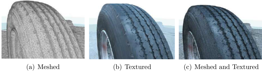
Figure 7.3: The profile obtained using the Fringe Projection Method (FPM) on a trailer tire Michelin 315/80R22.5 [MAN 19b].
