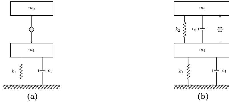
**Figure 1.19:** A SDOF primary system controlled by: (a) an AMD; (b) an ATMD.
