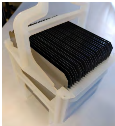
Figure 3.2. Teflon™ carrier containing the 25 as-cut wafers to be chemically etched
