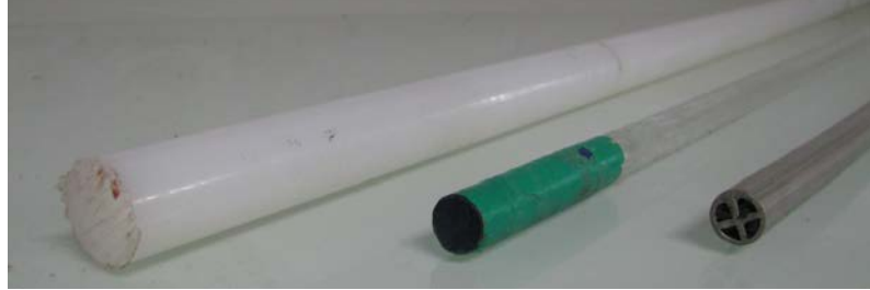
FIGURE 2.6: Nylon, PMMA, PVC striker bars
