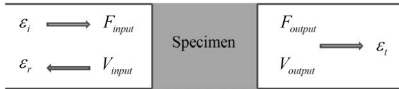
FIGURE 2.3: SHPB measuring technique
