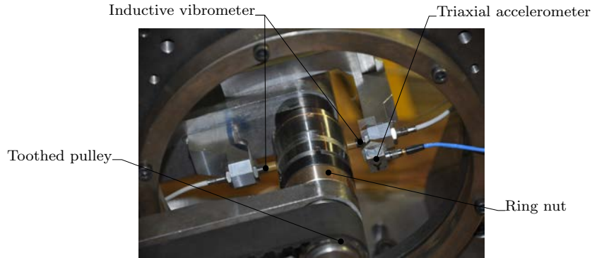
Figure 4.8: Acquisition sensor placement for squeal measurement.
