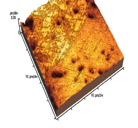
Roughness inside the wear track = Roughness outside
