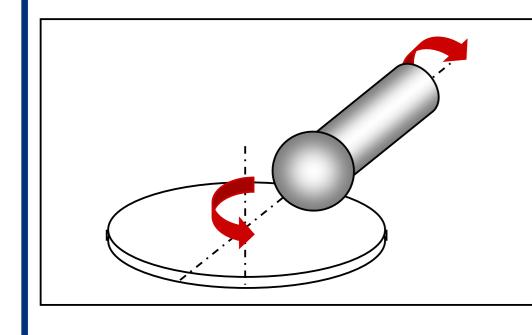
SRR\*\* <1, 1, 5 and 25% Mean Speed = 100 mm/s; Temperature =  $80^{\circ}$ C; Max Hertz Pressure = 890 MPa; Minimum film thickness= 11nm λ=0.95; 5h
