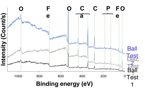
The same chemical components are detected in the rolling track on : Two balls from 2 different tests
