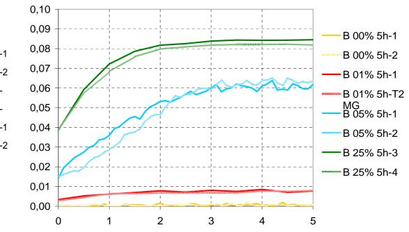
Friction coefficient increases when additives are present in the base oil Friction coefficient increases when SRR augments
