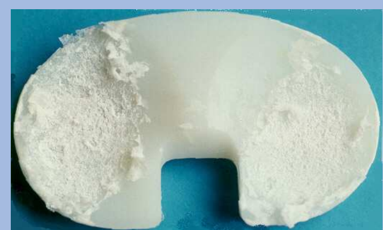
Friction surfaces wear
