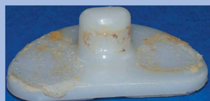
Loosening induced by small deflections at the bone / implant interface
