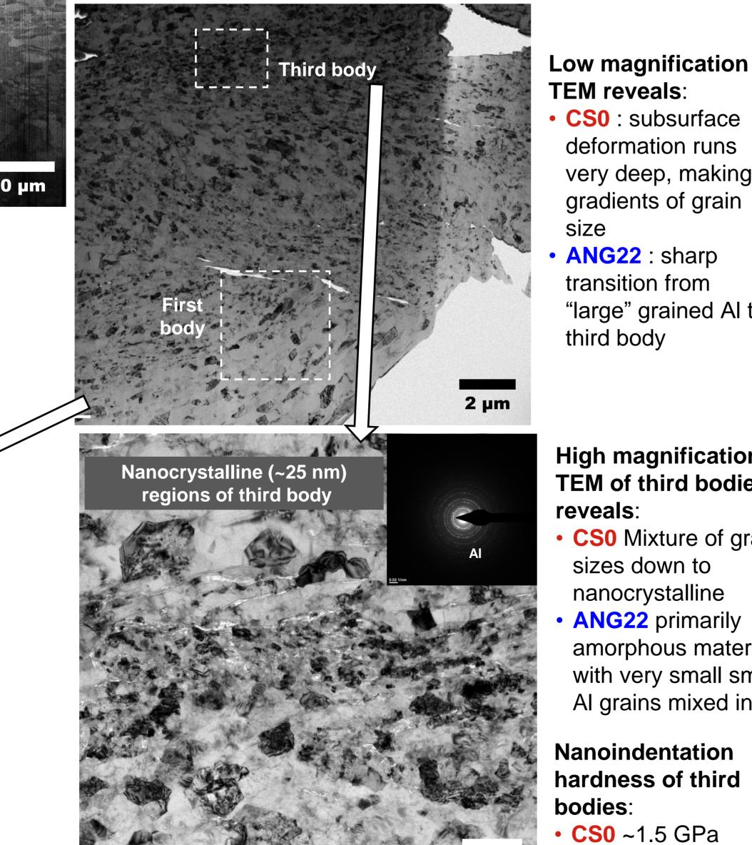
Surface analysis of wear tracks reveals: **CS0** shows evidence of adhesion and smearing ANG22 forms smooth, coherent tribofilms
