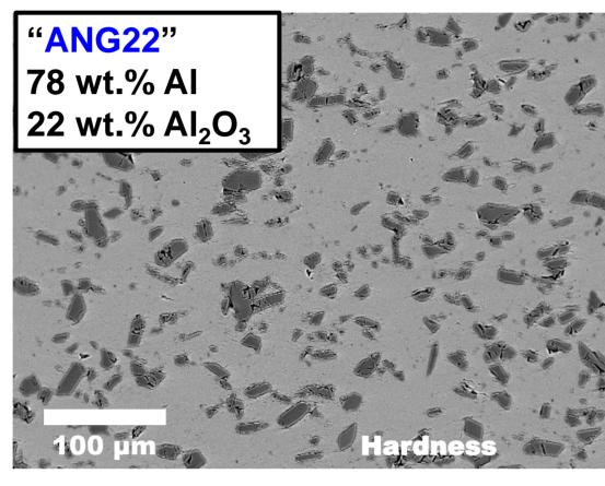
A proportion of the  $Al_2O_3$  particles were recovered to form a uniform  $AI-AI_2O_3$ microstructure.
