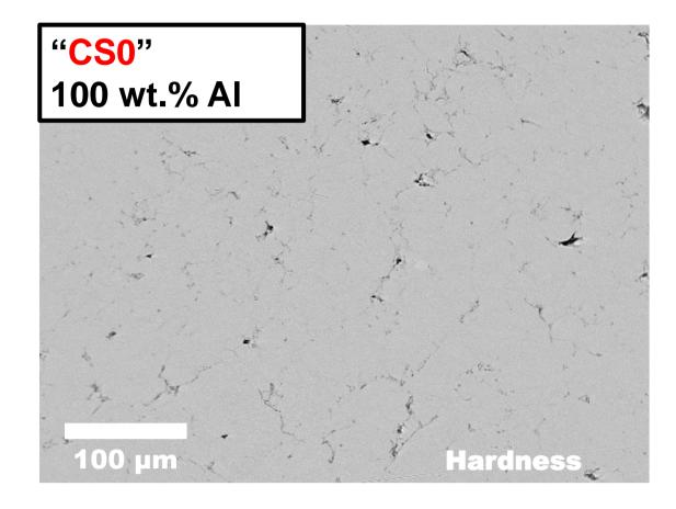
The pure AI coating consolidated into a dense microstructure with <2% porosity.
