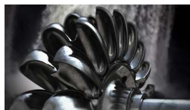
Figure 1.3: The blades of Pelton turbine.
