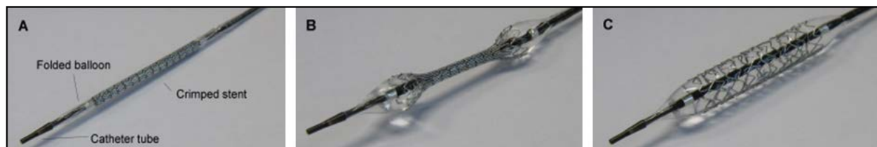
Figure II.5-1: Unconstrained expansion of the endeavor stent (Medtronic): (A) shows the stent, crimped around a folded angioplasty balloon. The deployment starts at the stent ends (B) and continues towards the stent center (panel C).
