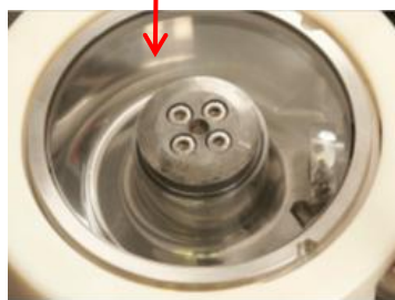
Figure 95: a) Picture of the JEROTRIB test-rig b) Zoom on the ball-on-disc part
