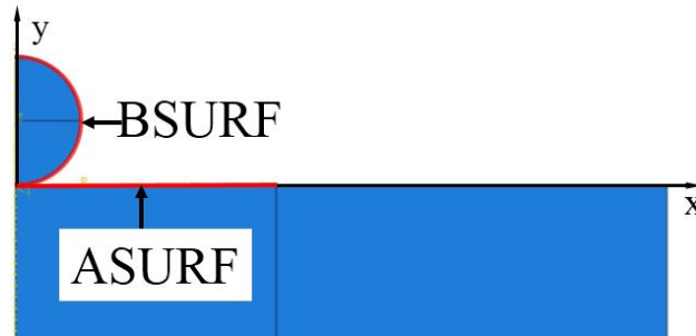
Figure 2.3: Schematic diagram of surface-to-surface contact.
