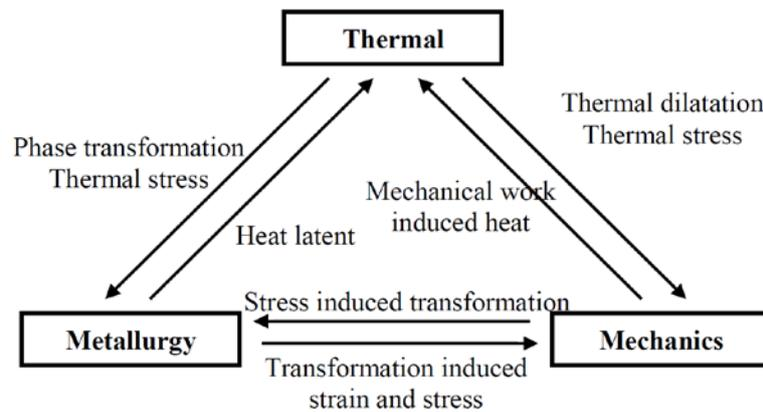
Fig. 1.2 Relation between Thermal, metallurgy and mechanics
