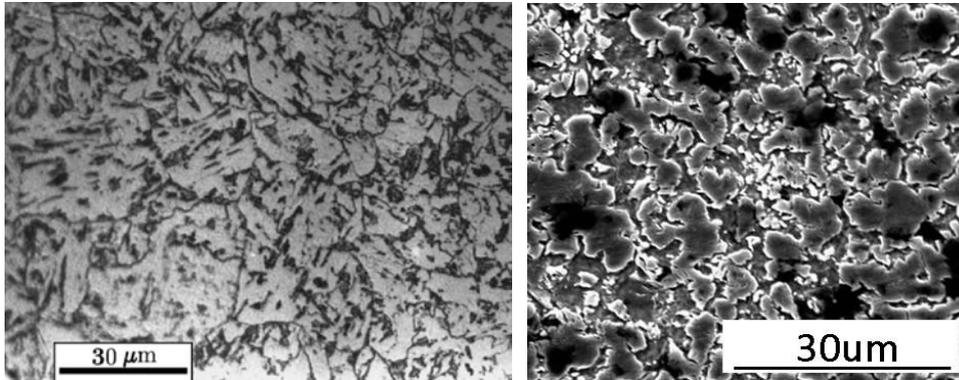
Fig. 5.32 Microstructure 16MND5 low carbon steel. The left one is the as-received condition [42] and the right one is the one after one cycle bainite transformation
