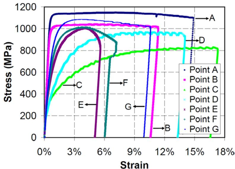
Fig. 4.7 Stress-strain curves of 15-5PH after different heat treatment history
