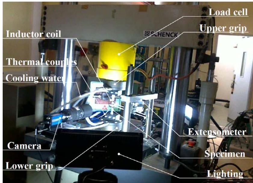
Fig. 4.4 Setup of devices for fracture test
