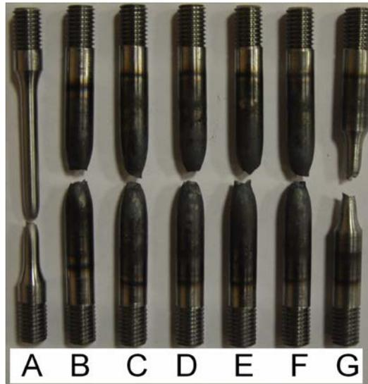
Fig. 5.26 Round bar samples after rupture
