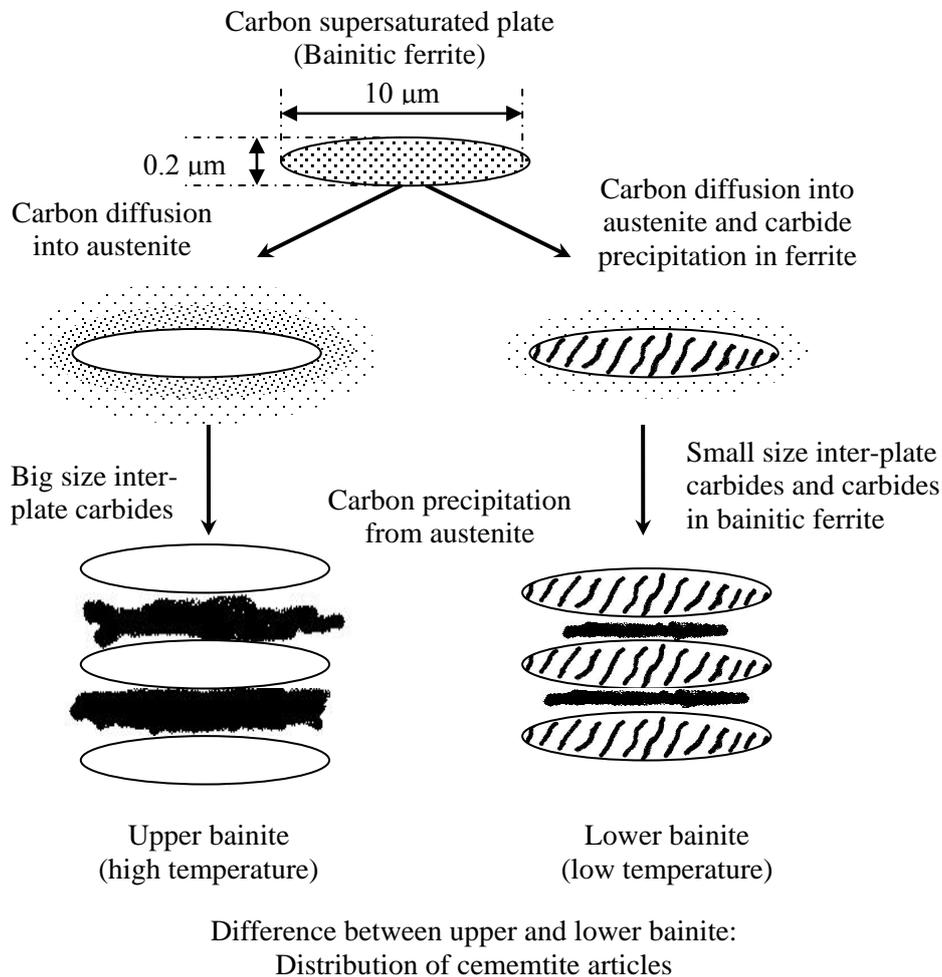
Fig. 2.20 Illustration of bainite transformation mechanism [65]
