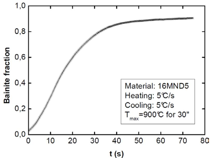
Fig. 2.22 Bainite fraction transformed during the continuous cooling bainite transformation
