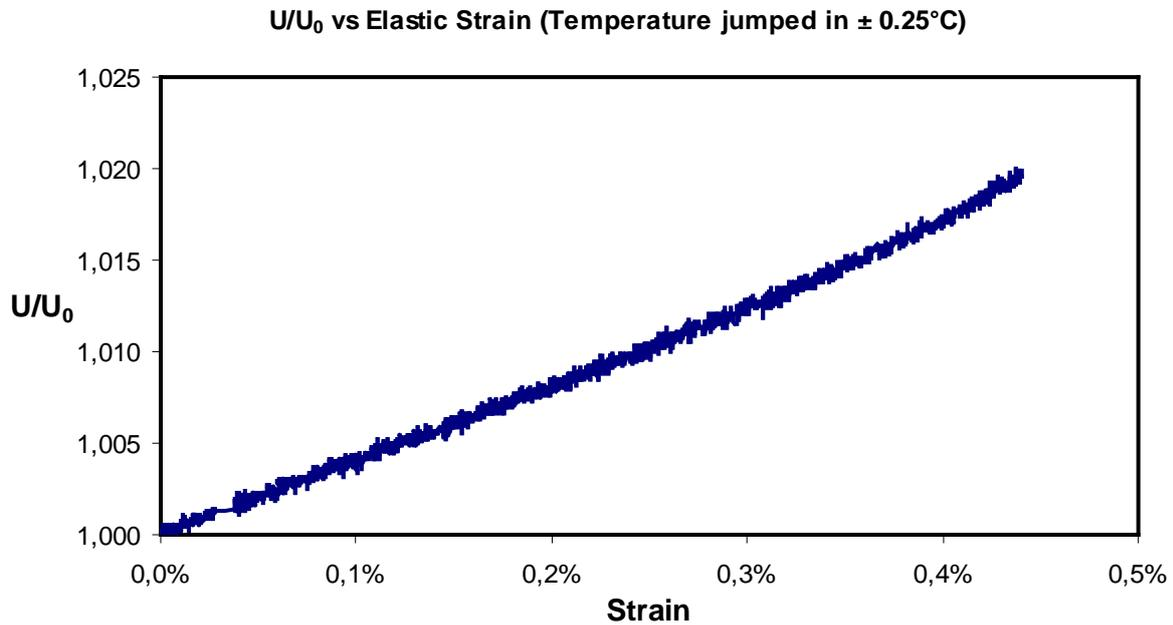
Fig. a13 Elastic strain induced potential drop
