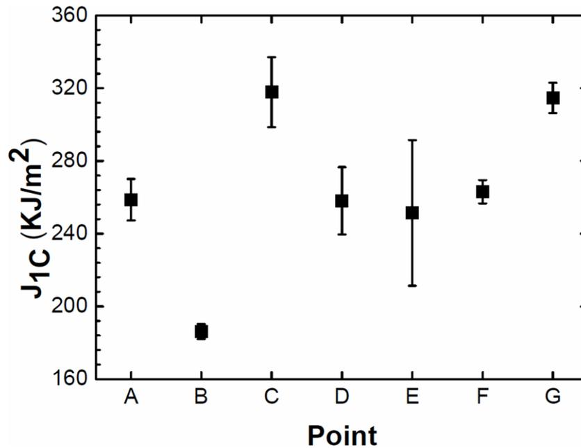
Fig. 4.12  $J_{1C}$  of 15-5PH at different temperature
