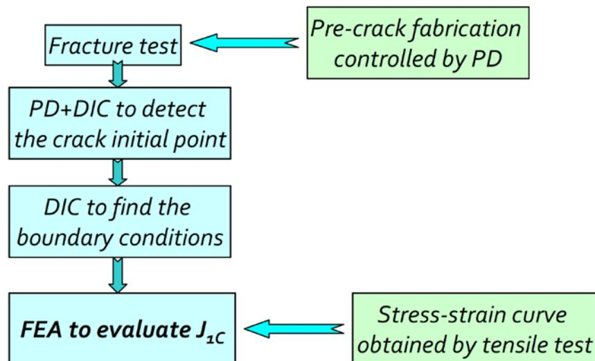
Fig. 1.3 Methodology to get  $J_{IC}$  from experiments
