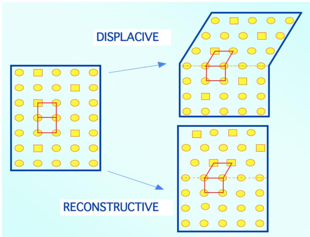
Fig. 2.10 The displacive and reconstructive mechanisms [34]
