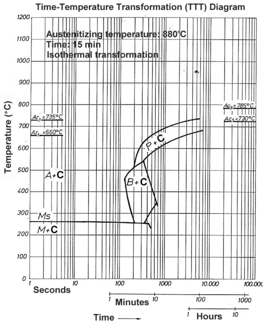
Fig. 2.12 TTT Diagram of 80WCrV8 alloy steel [37]
