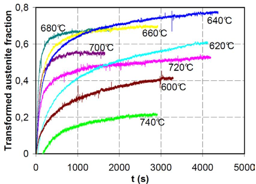
Fig. 5.10 Transformed austenite fraction versus time in the isothermal transformation before CCT Bc
