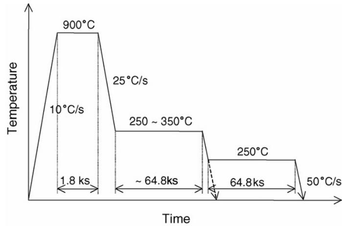
Fig. 2.28 The form of the 2-stage heat treatment
