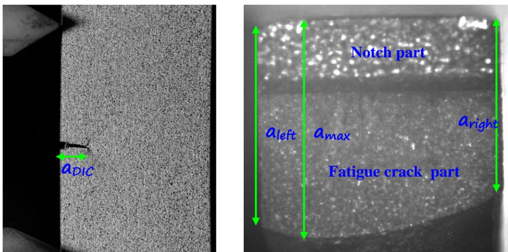
Fig. a8 The two “optical” crack length estimations: the left photo shows the DIC image used for initial crack length estimate  $a_{DIC}$ , the right one is the fatigue crack surface through the specimen observed after failure on which initial fatigue crack is easy to “see” with the microscope.
