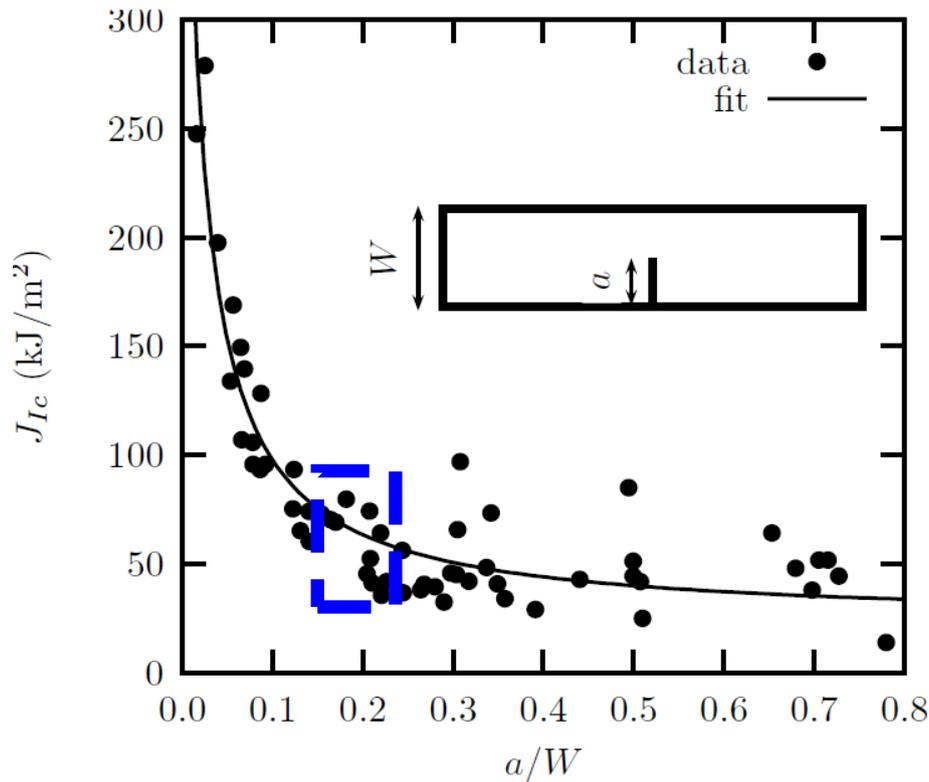
Fig. 3.16 Relation between  $J_{IC}$  with the pre-crack length [146]
