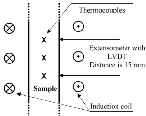
Fig. 4.5 Position of thermocouples and induction coil devices for mechanical tests
