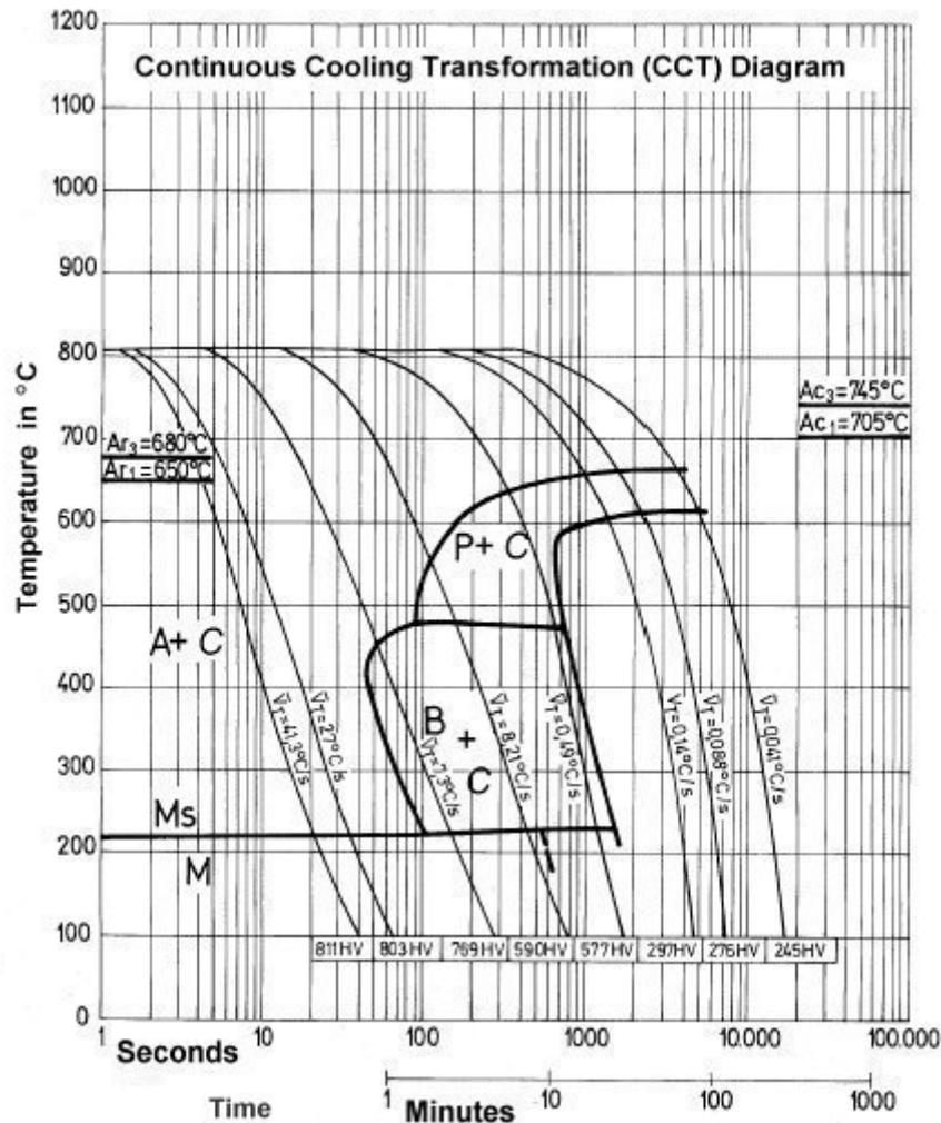
Fig. 2.11 CCT Diagram of one high carbon steel [36]
