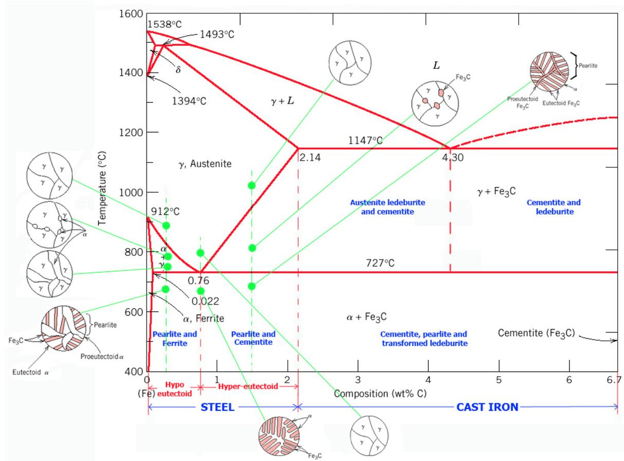
Fig. 2.8 Fe-Fe<sub>3</sub>C phase diagram [30]
