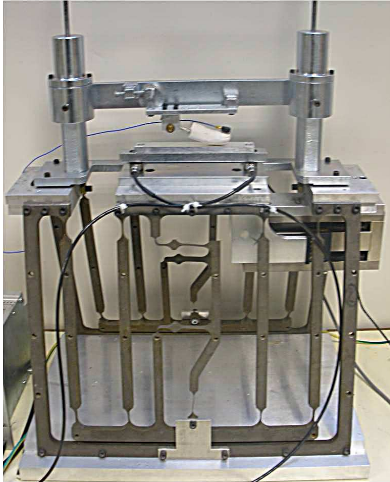
Figure 2.12: Tribotouch with the finger model (scale 1:4).
