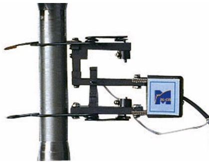
Fig. 2.9 Extensometer attached to a tensile test specimen
