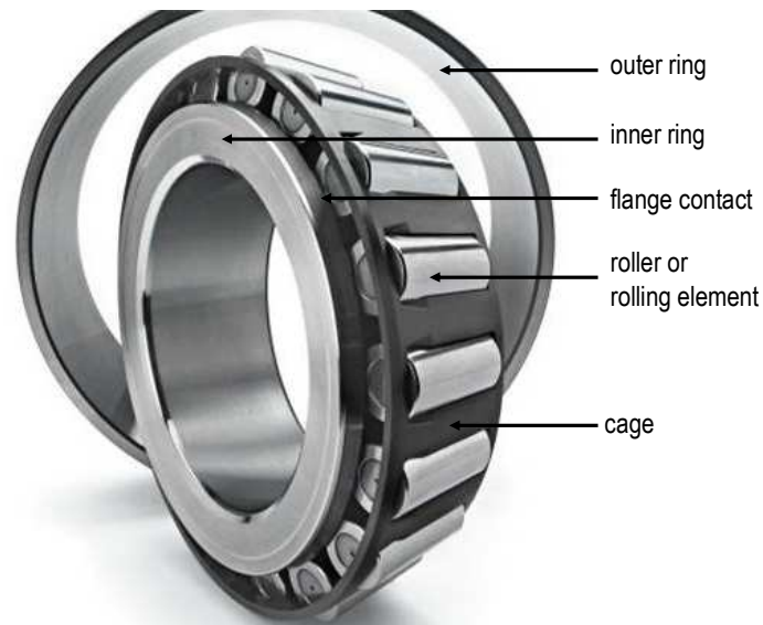
Figure 1.1 Tapered roller bearing (source: SKF)
