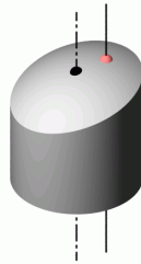
Figure C.2 Schematic showing unwanted eccentricity of the spherical-end specimen
