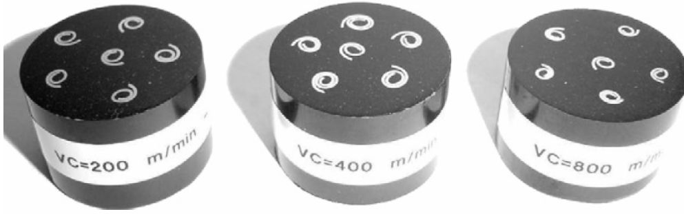
Fig. 2.12 Chips embedded in resin ( f = 0.4 mm/rev, V_C = 200, 400 and 800 m/min)
