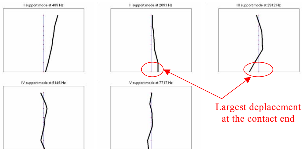
Figure 4.4 Tangential modes of the support in the frequency range of interest. The blue line is the undeformed grid of the cylindrical body of the support; the black line is the deformed shape.
