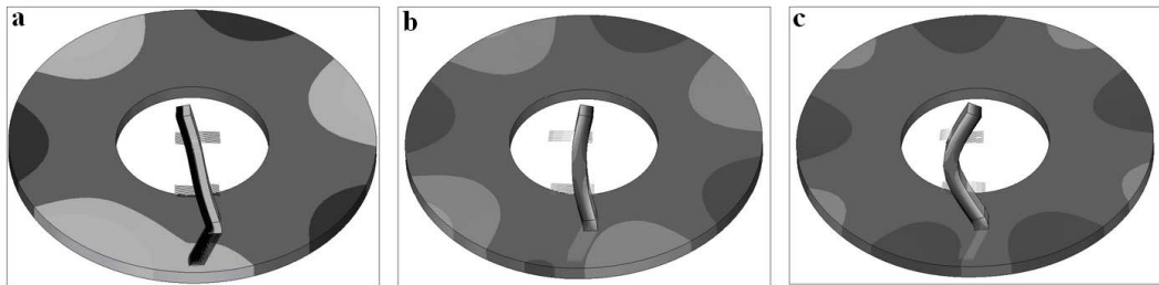
Figure 3.11 Unstable modes computed for a friction coefficient equal to 0.5: a) Unstable mode at 3 kHz ( 10^{9.6} Pa); b) unstable mode at 3.5 kHz ( 10^{10.6} Pa); c) unstable mode at 5 kHz ( 10^{10.6} Pa).
