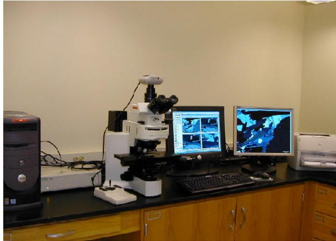
Figure A. 5 *Optical microscopy (ZEISS AX10PHOT)*
