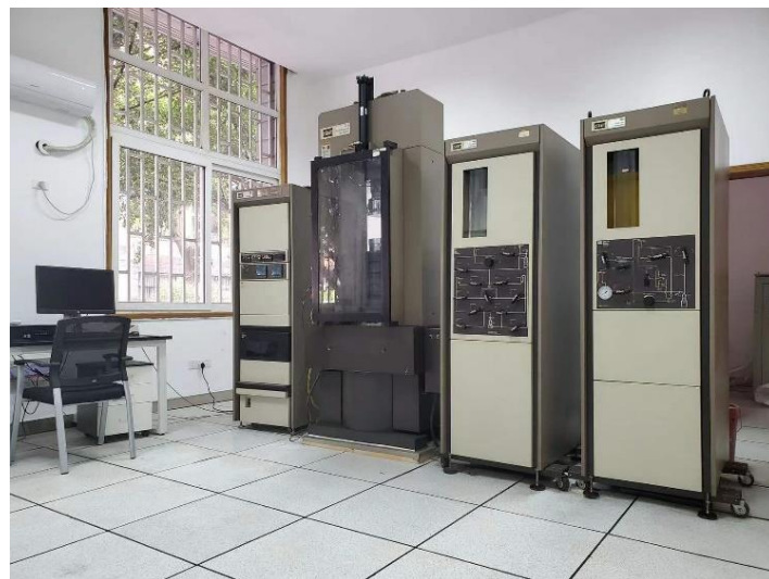
Fig. 2.5 The MTS 815 rock mechanics test system used in this experiment
