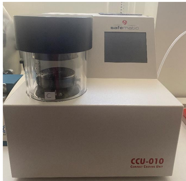
Figure 3.12: CCU-010 Compact coating unit for carbon layer deposition
