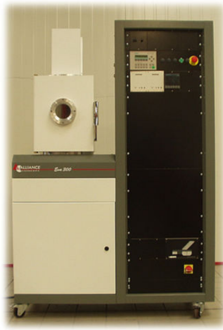
Figure 4.7: EVA300 vacuum evaporation machine.
