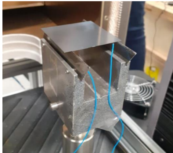
Figure 4.11: Silicon sample positioned on the 4-line bending apparatus before testing.
