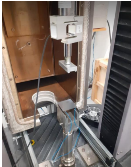
Figure 4.6: Four line bending mechanical test.
