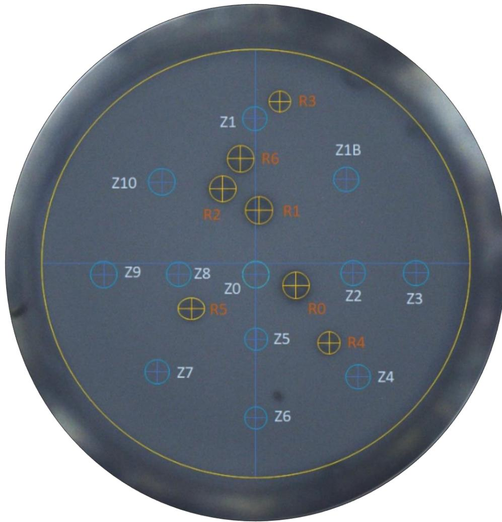
Figure 4.1 : Microscope image taken with the VIPA set up of the DAC, loaded with ruby microspheres (black point) immersed in squalane at ambient conditions. The yellow circles indicate the ruby sphere's location, blue circles the locations where the Brillouin spectra were taken. The outer circle represents the boundaries of the 200 μm hole inside the steel gasket.
