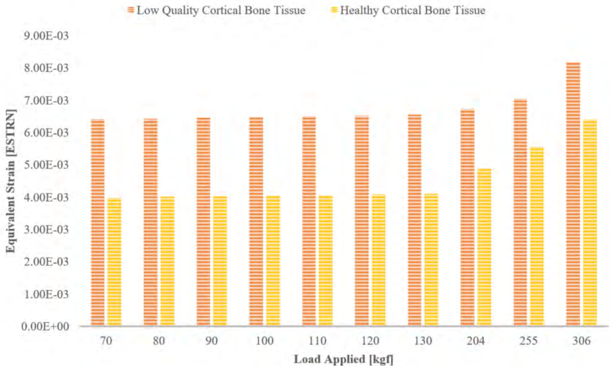
Figure 4.58. Maximum strain results of the femur and custom hip stem assembly
