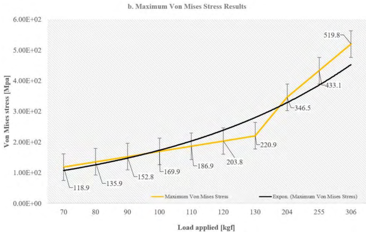
Figure 4.6. Minimum and maximum Von Mises Stress results [MPa] obtained in case of the pelvis CAD model
