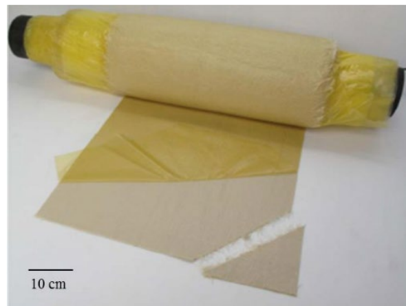
Figure 1.14. Photograph of a roll of glass-fibre SMC prepreg (Ferré Sentis, 2017).
