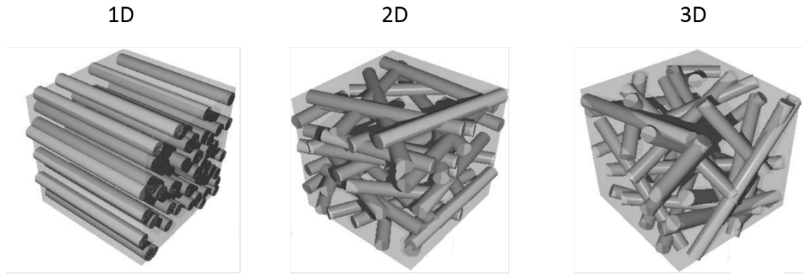
Figure 2.6. Numerically generated virtual fibrous networks with (i) aligned fibres in one direction (ii) 2D random and (iii) 3D random fibre orientations (Tomadakis et al., 2005).
