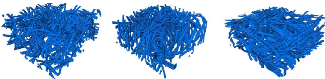
Figure 2.8. Examples of 3D microtomography images of fibre mats that exhibit different fibre orientations (Soltani et al., 2014b)
