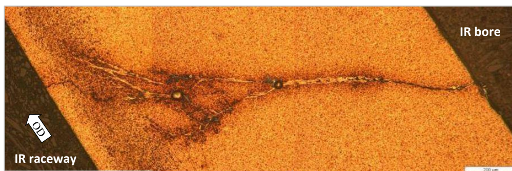
Fig. 4.20: Circumferential LOM of a specific NTN-SNR DGBB IR tested on a Machine S with highly additivated lubricant B: WEA form aside cracks that initiated at the IR bore due to intense fretting.
