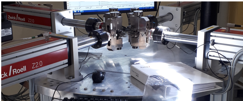
FIGURE 3.9 – Machine de traction biaxiale Zwick
