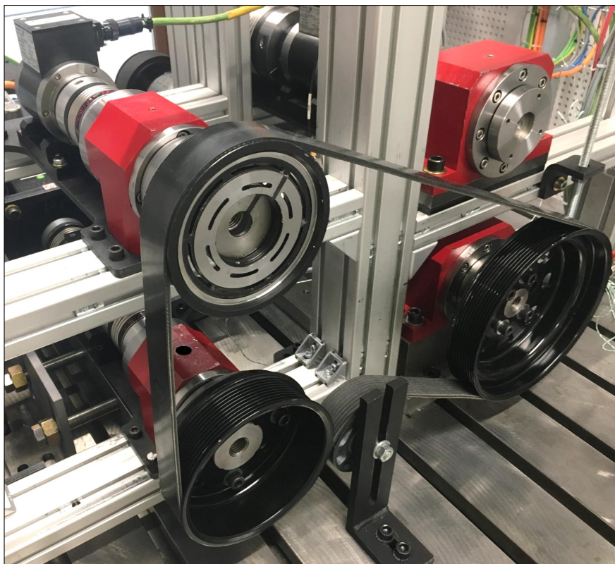
Figure 4.7 – FEAD case study used to validate the optimization of PL_{FEAD} .
