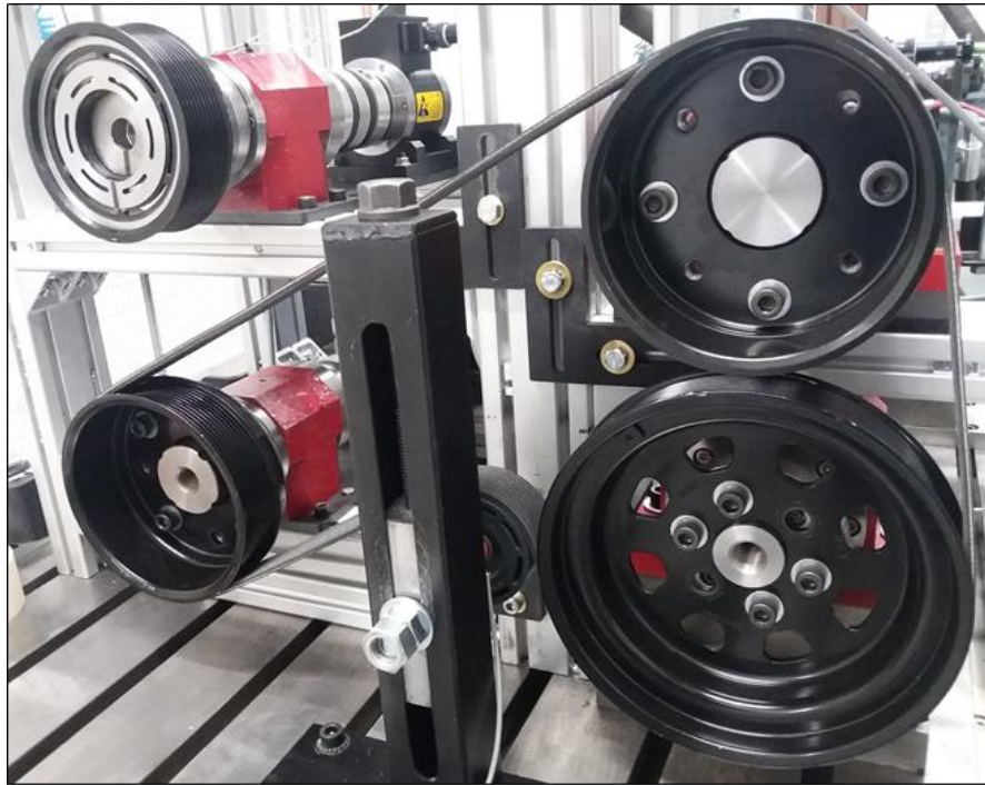
Figure 4.6 – FEAD case study used to validate the modeling of PL_{FEAD} .
