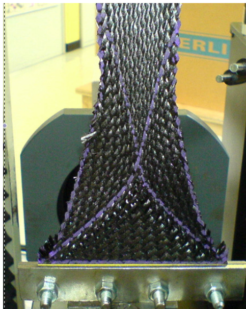
Figure 9: Shear behavior in the plane of the yarns of fibrous composite reinforcements.
