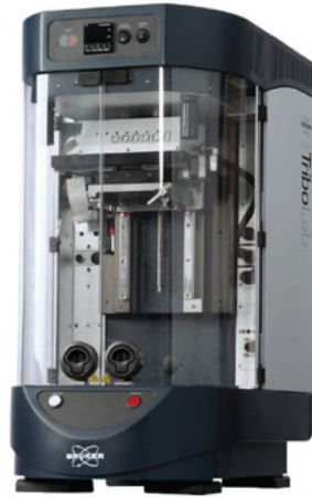
Figure 5.1: Bruker UMT Tribolab
