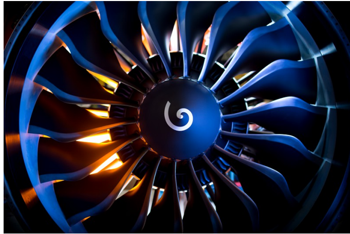
Figure 1.4: LEAP fan blades in RTM woven composite materials.
