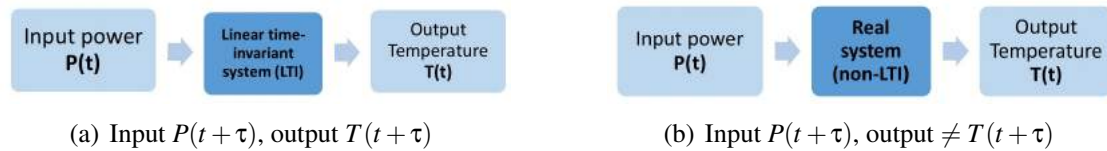
Figure 5.4: Difference in temporal respond between LTI system and non-LTI system
