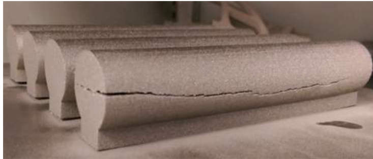
Figure 1.10: Crack caused by residual stress[COM 17]
