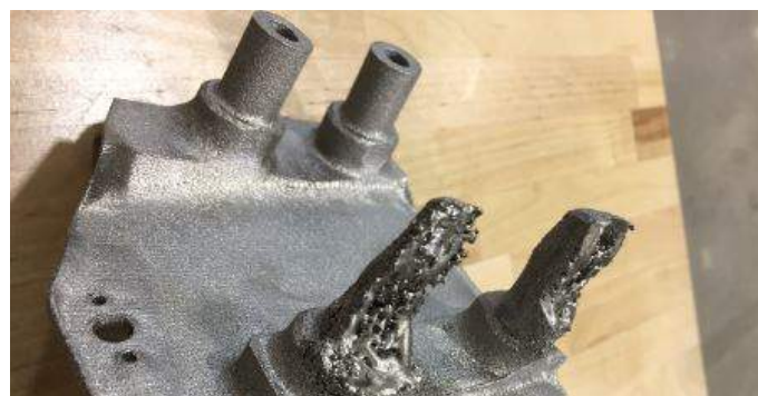
Figure 1.16: Incompleted parts induced by lack of fusion[MCG 17]
