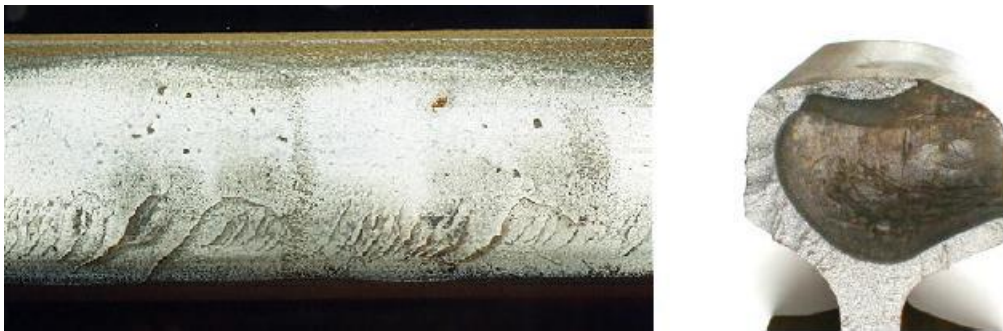
Figure 31 Severe Head Check sur rail (Dollevoet, 2010)
