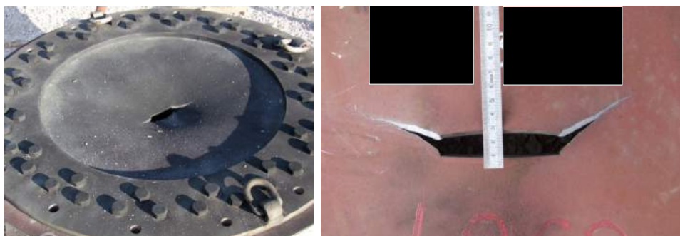
FIGURE 3.49: Tir T3 - x kg - 2D mm - Préfissure 80mm [DCNS].
