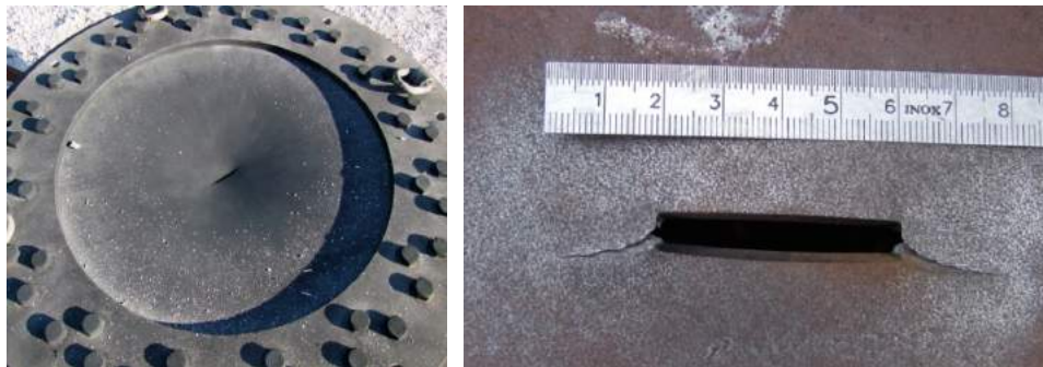
FIGURE 3.47: Tir T1 - x kg - 2D mm - Préfissure 40mm [DCNS].
