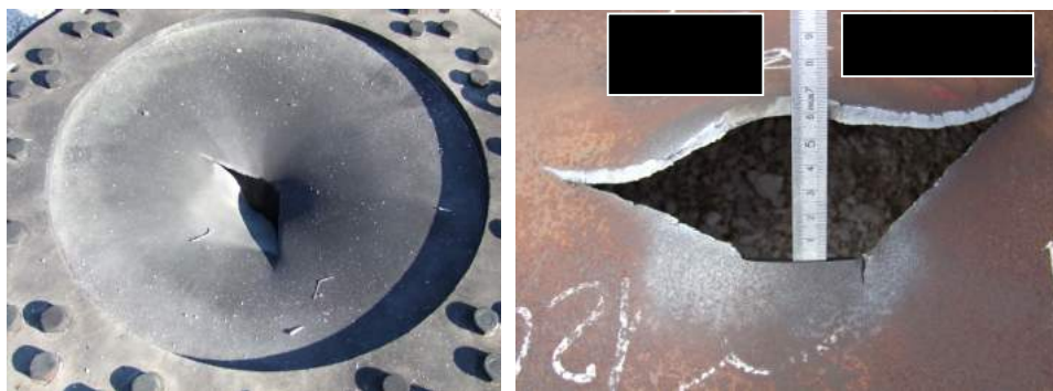
FIGURE 3.48: Tir T2 - x kg - D mm - Préfissure 40mm [DCNS].
