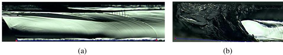
**FIGURE 3.12:** Two different precrack front shapes in accordance with the two precracking strategies. Crack propagation  $< 2900\text{m/s}$  initiates from long elliptical precrack (a) and crack propagation  $> 2900\text{m/s}$  starts from short straight precrack (b). The dimension can be referred to the specimen's thickness *i.e.*  $190\ \mu\text{m}$
