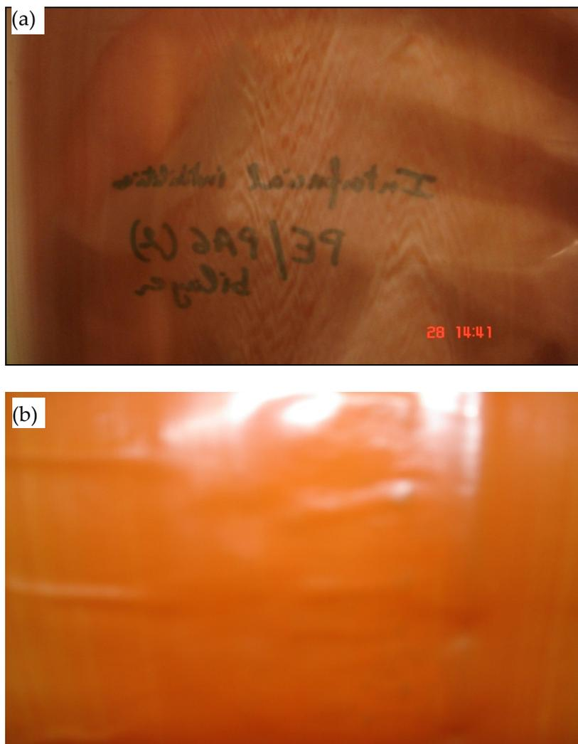
**Figure I- 27** Photographs of (a) the instabilities in the case of the PA6 (2)/PE bilayer system observed at  $T = 240^{\circ}\text{C}$  with a coat hanger die and a flow rate ratio equal to 1 ( $Q_{\text{PA6}(2)} = Q_{\text{PE}} = 2 \text{ kg/h}$ ); (b) a stable bilayer system based on PEGMA/ PA6 (2) obtained under equivalent conditions. (The red pigmented sample correspond to PE-GMA and PE). (from Lamnawar and Maazouz 2009)
