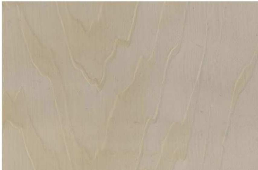
**Figure I- 24** An example of a wavy interface observed in a PVDF/PE bilayer film
