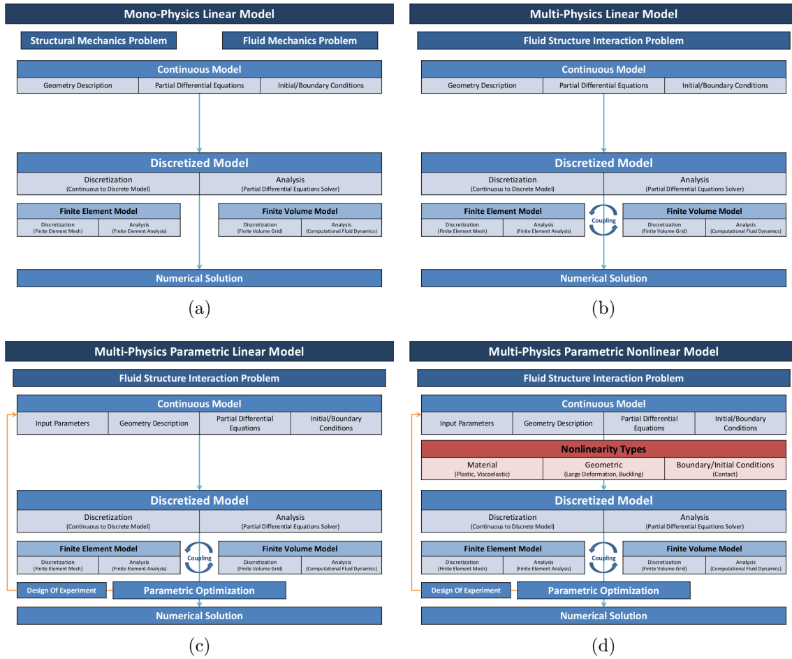
Figure 1.3: Different types of numerical models with increasing complexity: Mono-physics linear model (a); Multi-physics linear model (b); Multi-physics parametric linear model (c); Multi-physics parametric non-linear model (d).
