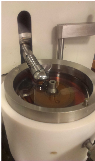
FIGURE 4.5: La machine MTM (Mini Traction Machine) [ http://pcs-instruments.com/ ].
