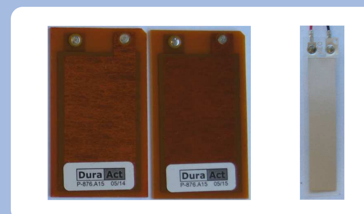
Figure 4. Actuators and sensors
