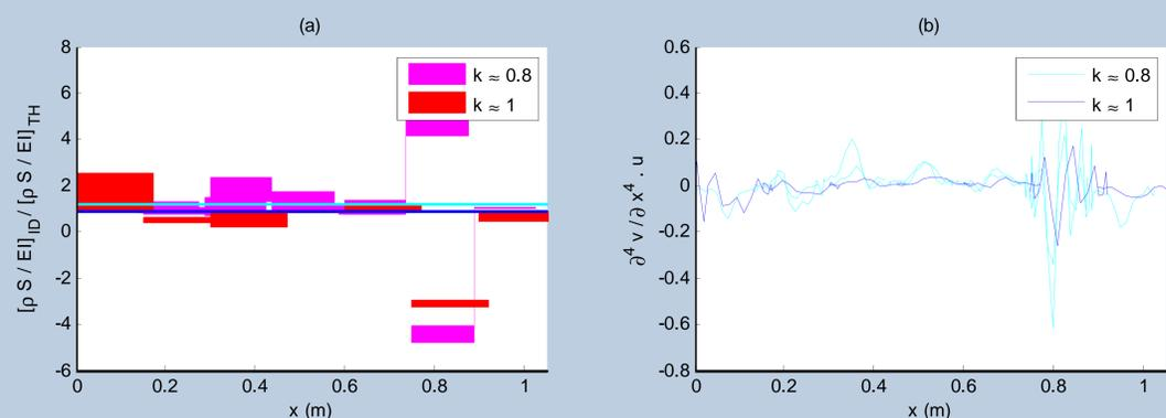
These results demonstrate an alternative method for damage location. Indeed, with a restricted number of samples, it was shown that  $\rho S/EI$  and the fourth derivative  $\partial^4 v / \partial x^4$  can be computed. The parameters studied are very sensitive to damage (a discontinuity).  $\rho S/EI$  becomes negative when the continuity assumption is no longer valid. The damage can also drastically increase the  $\rho S/EI$  value.
